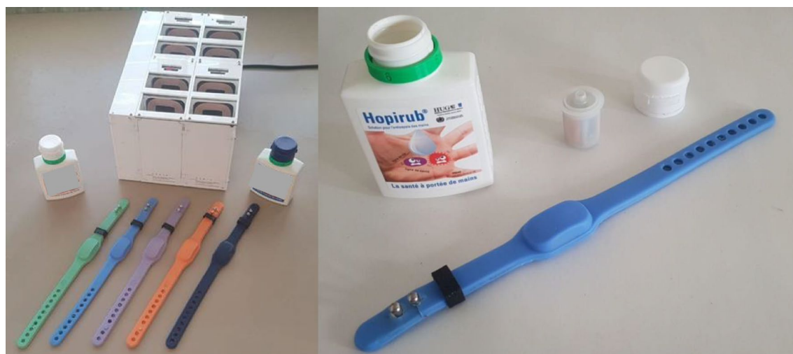
Fig. 1 Three hardware components of SmartRub ® device: the station, the bracelet and the cylinder
